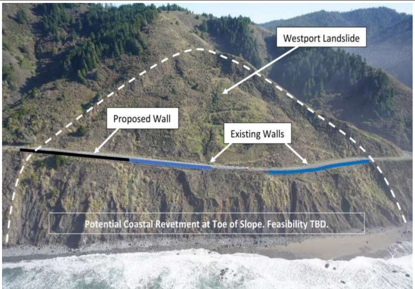
The Westport Slide Project is Back! This map shows the location of proposed SPGA wall and revetment feasibility at the toe of the slide (courtesy of Caltrans).
