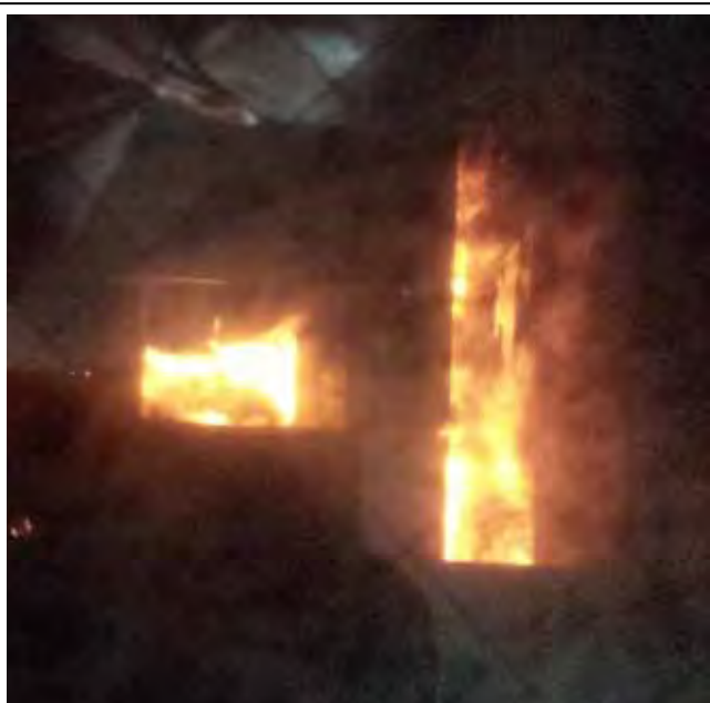
Inside the burning trailer during a flashover
